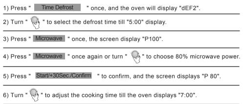
7) Press "Start/+30Sec./Confirm" to start cooking, and buzzer will sound once for the first section, defrosting time counts down; buzzer will sound once again entering the second cooking. when cooking finish, buzzer sounds five times.
